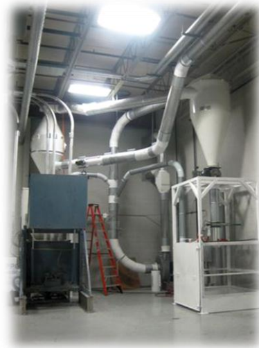
Elutriation System, Dust/ Good Product Separation from Regrind at Extruder
