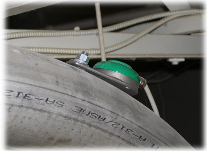
Acoustic and Microwave Plug Chute and Automatic Blower Shutdown Sensors
